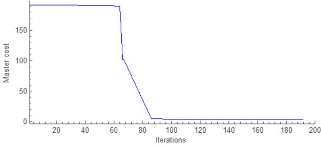
Fig. 3. Improvement in the master cost during optimization starting from initial parameter values  $[w_p \ w_v \ w_w] = [10000 \ 10000 \ 1000]$ .
