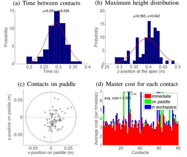
Fig. 5. Results for 3 parameters with average cost 4.503; parameters set to  $[w_p \ w_v \ w_w] = [9331.227812 \ 336.372829 \ 5758.953800]$  with  $|u_{max}| \leq 25$ .
