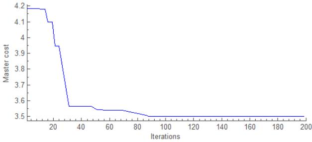
Fig. 6. Improvement in the master cost during optimization starting from initial parameter values  $[w_p \ w_v \ w_w] = [10000 \ 100 \ 1000]$ .
