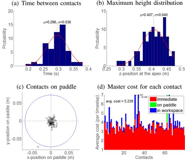
Fig. 2. Results for initial parameters with average cost 5.239; parameters set to  $[w_p \ w_v \ w_w] = [10000 \ 10000 \ 1000]$  with  $|u_{max}| \leq 40$ .
