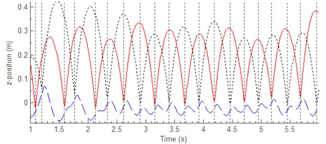
Fig. 9. Trajectories (z-coordinate) of the paddle (blue dashed) and the balls (red solid and black dotted).
